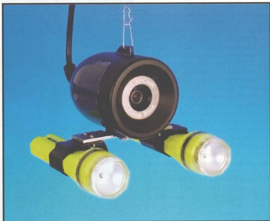
Splashcam Deep Blue Pro ready for deployment, with twin waterproof flashlights.
